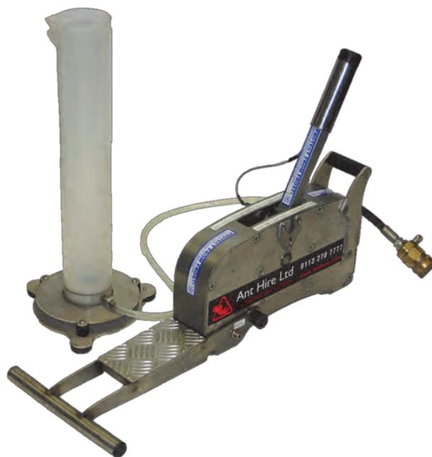
The machine has been created for carrying out hour-long pressure tests for ductile iron, PVC, GRP or stainless steel pipes. For this test type, a system test pressure (STP) needs to be maintained and the volume added, measured. The machine allows the water added to be accurately measured remotely, eliminating the possibility for human error.
